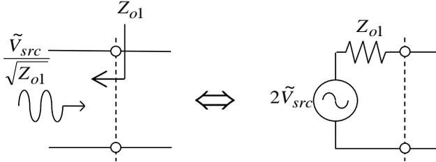
Figure 2.2. Thévenin equivalent circuit of the power wave source voltage.
