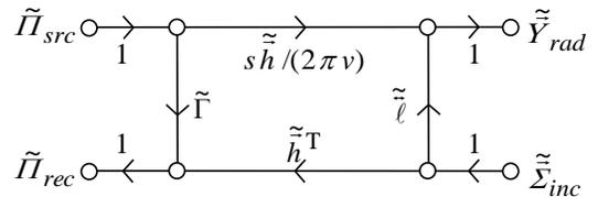
Figure 6.3 Vector signal flow graph representation of the GASM including both polarizations.
