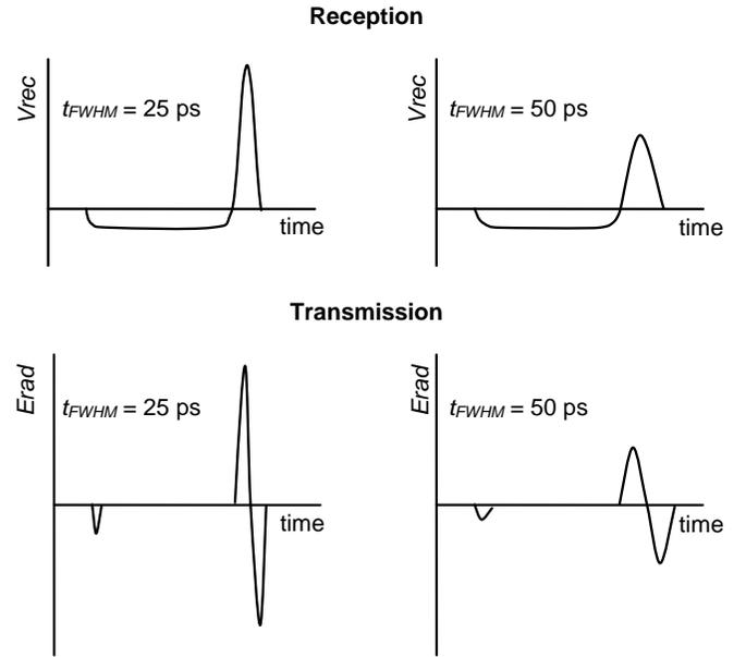
Figure 1.2. Characterizing an Impulse Radiating Antenna on boresight for dominant polarization by its response to an incident infinite plane-wave electric field with Gaussian time dependence (top), and a Gaussian 50- $\Omega$  source voltage (bottom), at two different Gaussian pulse widths (left and right). Note that  $t_{FWHM}$  is the Full-Width Half Max of the incident field or voltage. (Scale is approximate.)
