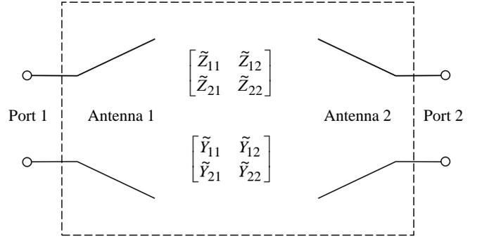
Figure 2.3. Two-port equivalent circuit of a two-antenna system.
