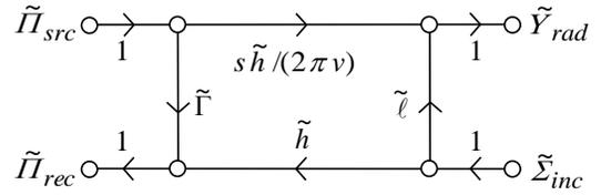
Figure 6.2 Signal flow graph representation of the GASM.
