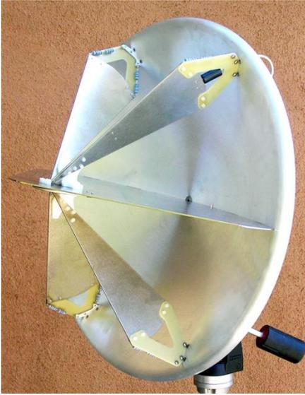
Figure 1.1. The Farr Fields model IRA-3Q, with a diameter of 46 cm.
