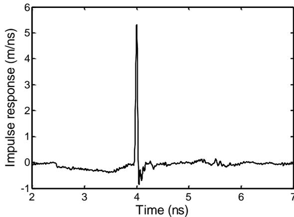
In Figure 9.1 we show the impulse response and transfer function on boresight for dominant polarization of the IRA-3Q shown earlier in Figure 1.1. This was measured on the Farr Fields time domain antenna range, using a Tektronix model TDS8000B sampling oscilloscope with a model 80E04 sampling head, a Picosecond Pulse Labs model 4015C pulser, and a Farr Fields model TEM-1 TEM sensor.
