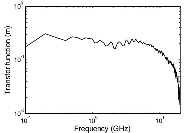
Figure 9.1. Impulse response (left) and transfer function (right) of the IRA-3Q.
