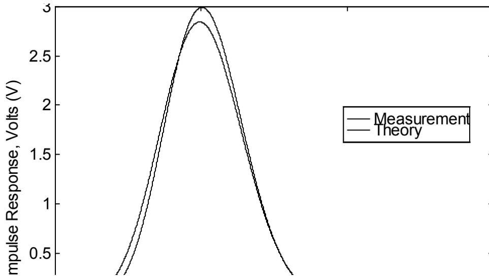
Figure 4.6. Impulse response for propagation through 7.16 cm of water.
