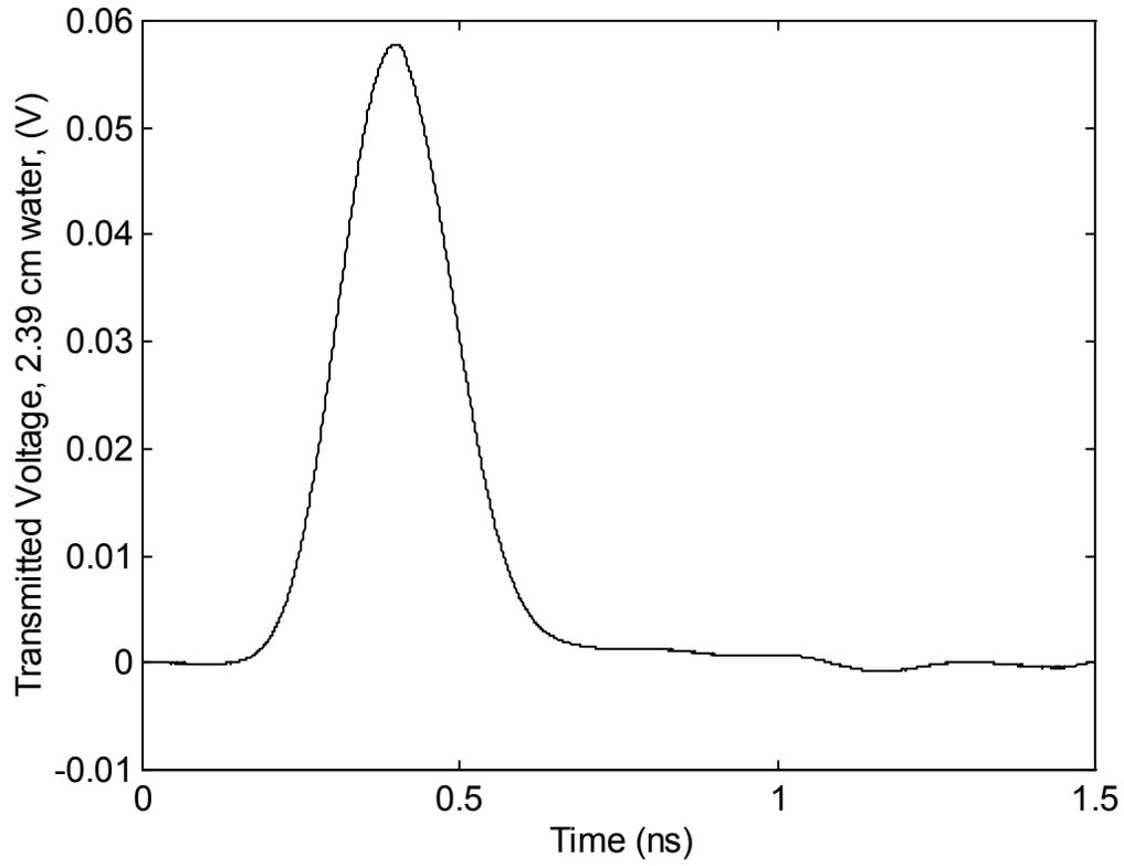
Figure 4.3. Signal transmitted through 2.39 cm of distilled water
