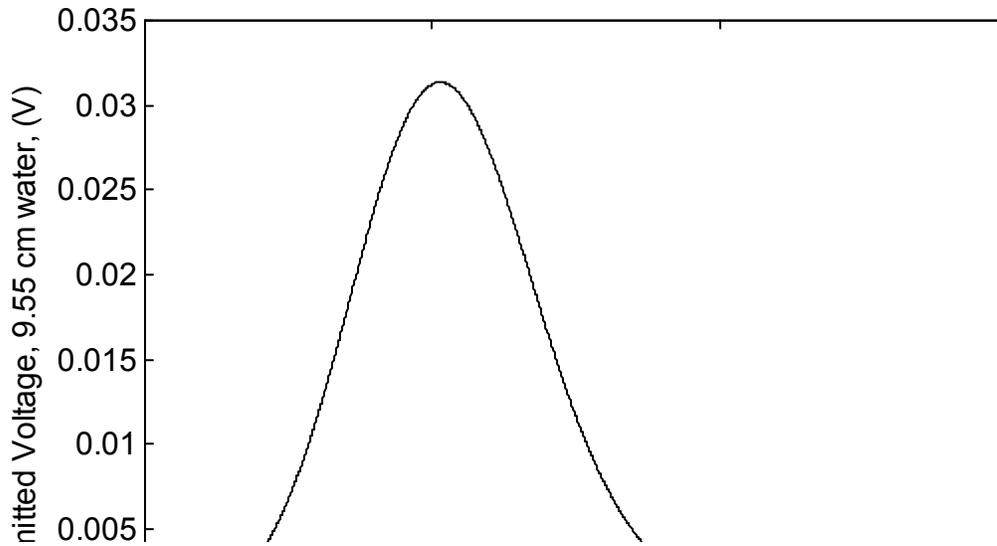
Figure 4.4. Signal transmitted through 9.55 cm of distilled water
