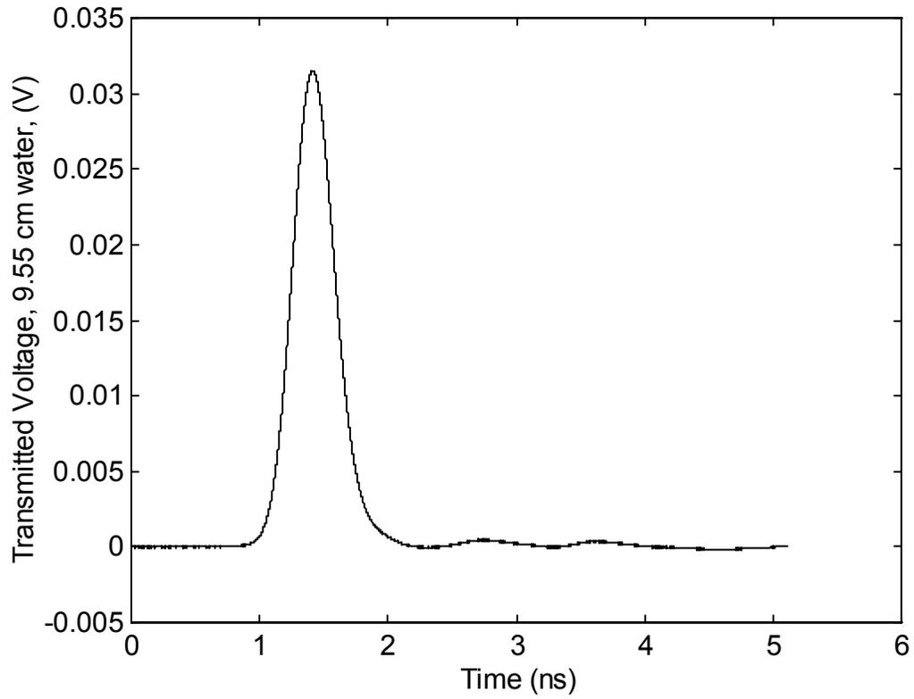
Figure 4.10. Signal transmitted through 9.55 cm of distilled water
