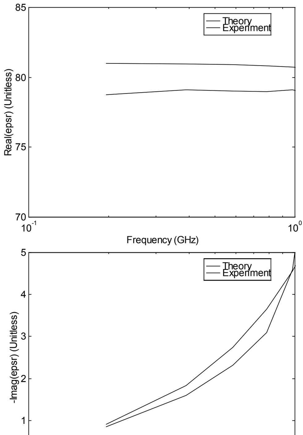
Figure 4.12. Real (top) and imaginary (bottom) parts of the measured dielectric constants of distilled water, using water columns 9.55 and 76.39 cm in length..
