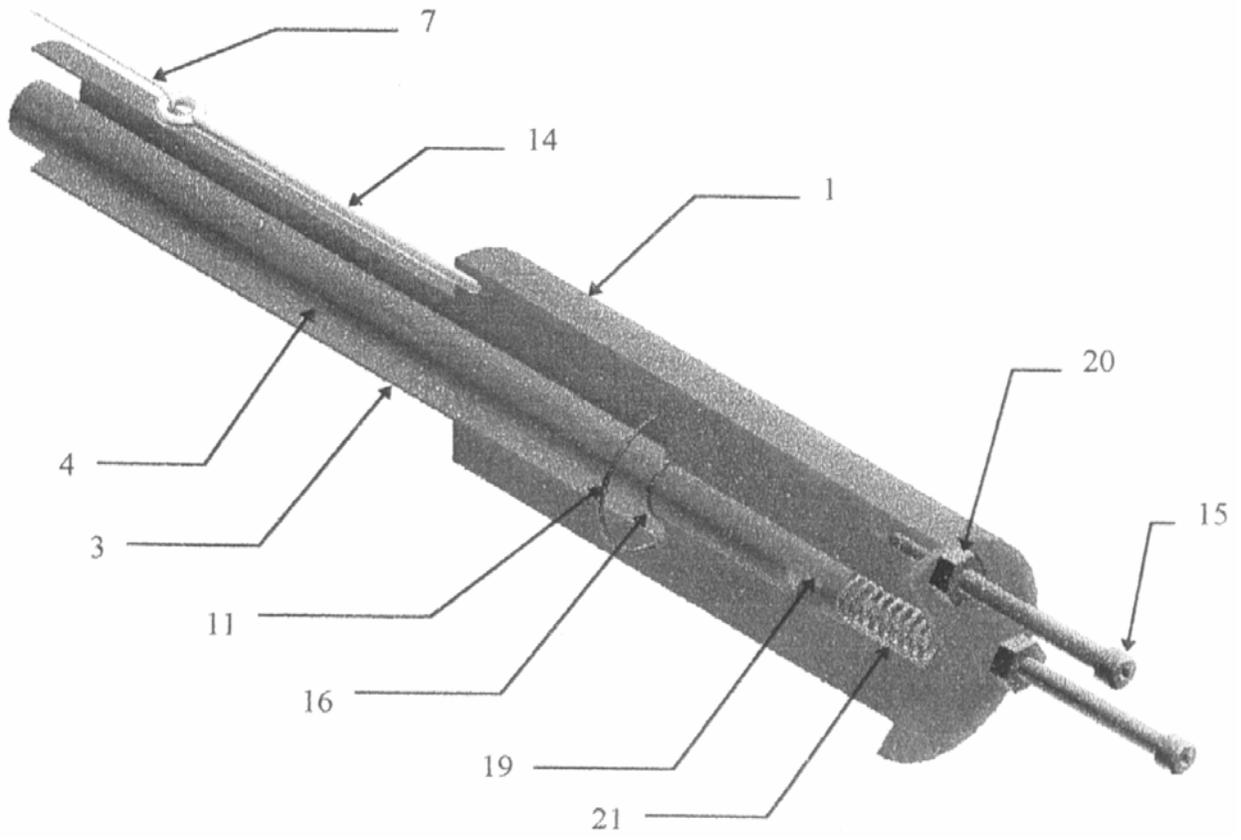
Figure 3.5. Planar short circuit.
