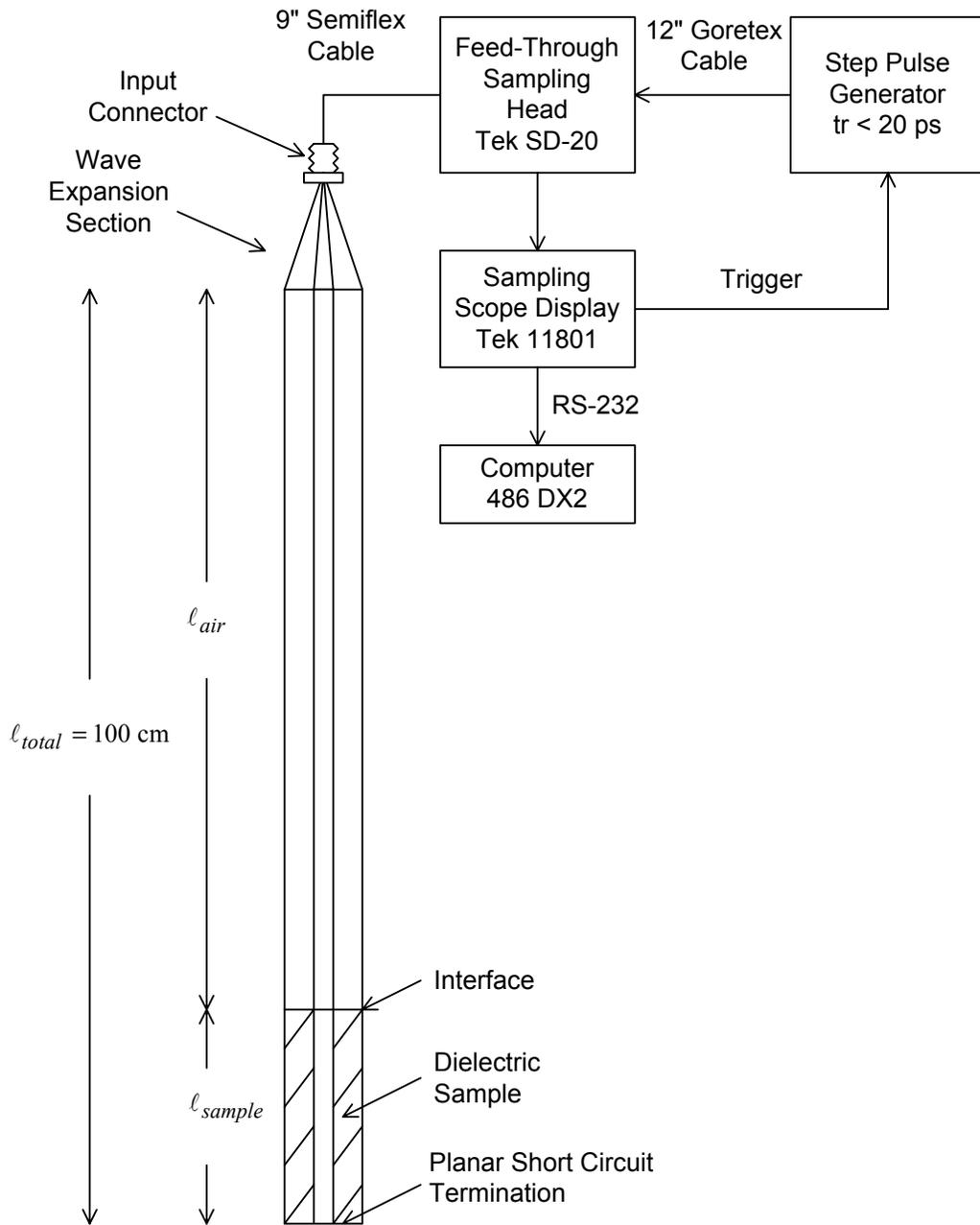
Figure 3.1. Instrumentation setup for measurements in TDR mode.
