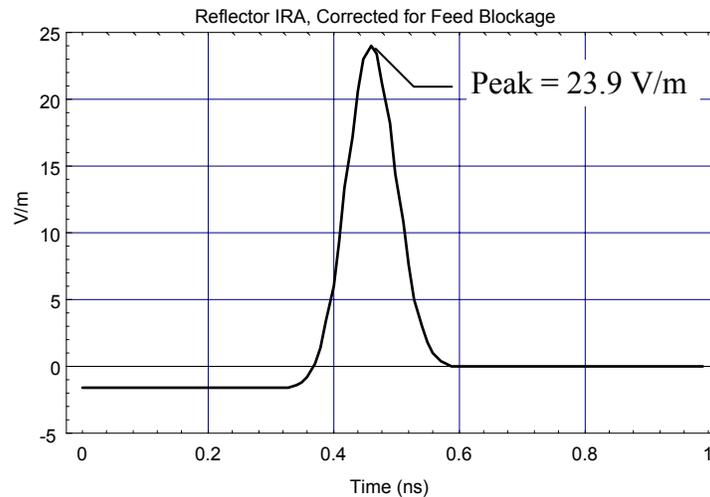
Figure 4.5. Reflector IRA predictions corrected for feed blockage.
