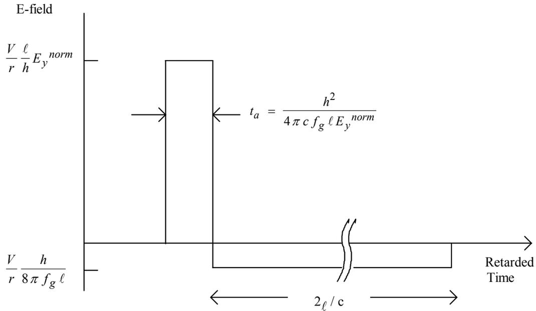
Figure 2.5. Approximate step response of a TEM horn.
