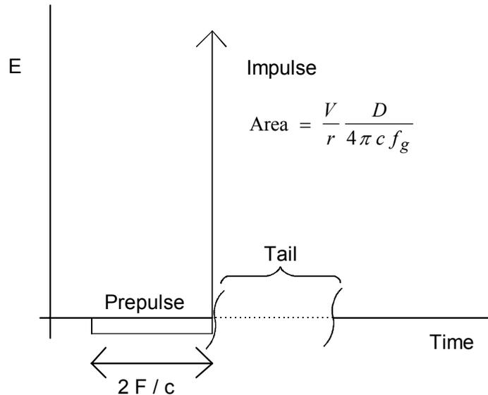
Figure 2.1. Step response of reflector IRA on boresight.
