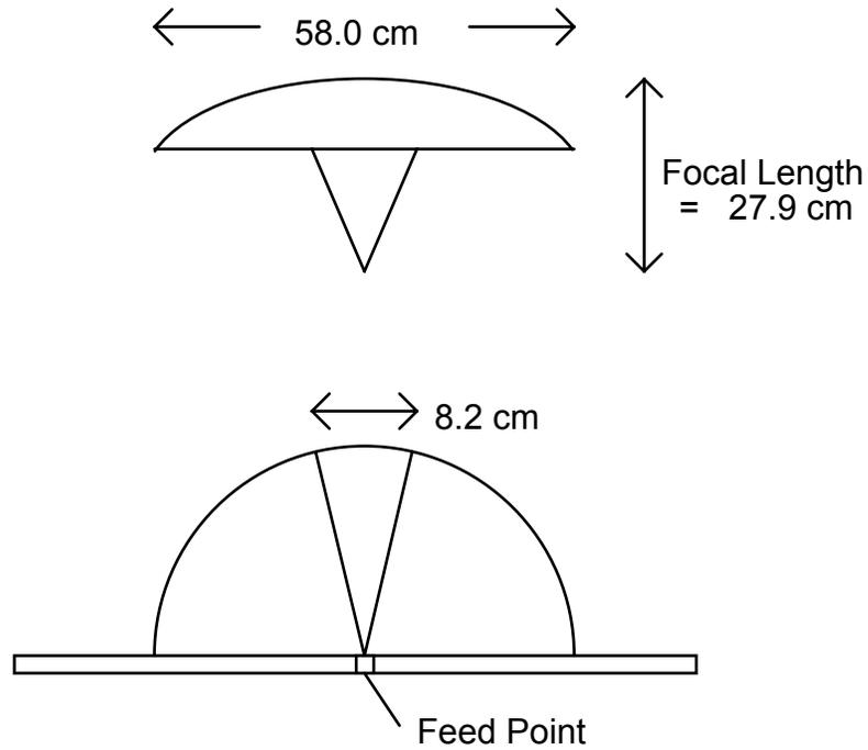
Figure 3.2. The reflector IRA studied in this experiment
