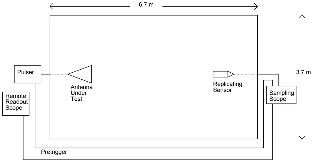
Figure 3.3. The experimental test setup
