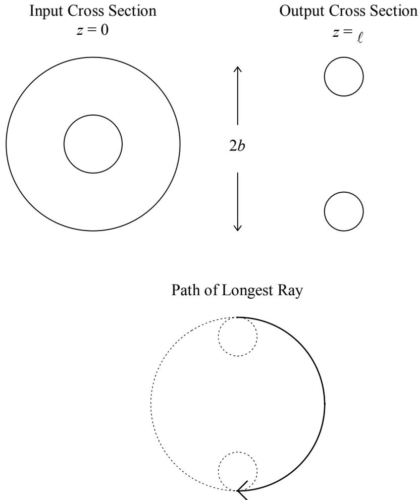
Figure 6.1. Geometry for tracing the longest path through a balun.
