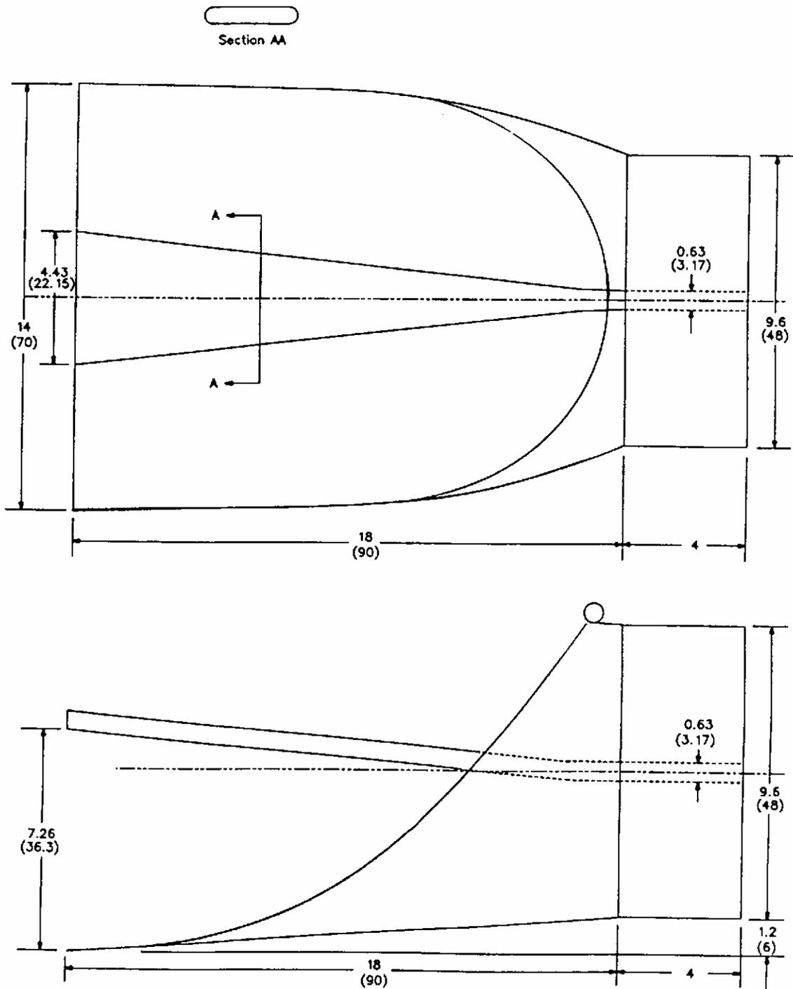
Figure 6.2. Transition section at ARES. Dimensions in parentheses are for the full-scale device as installed at ARES, in inches. Dimensions not in parentheses are for a one-fifth scale model, also in inches.
