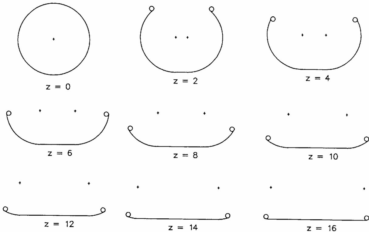
Figure 6.1. Unfolding of the ARES transition. Dimensions are in inches for a one-fifth scale model of the actual transition as built at ARES.
