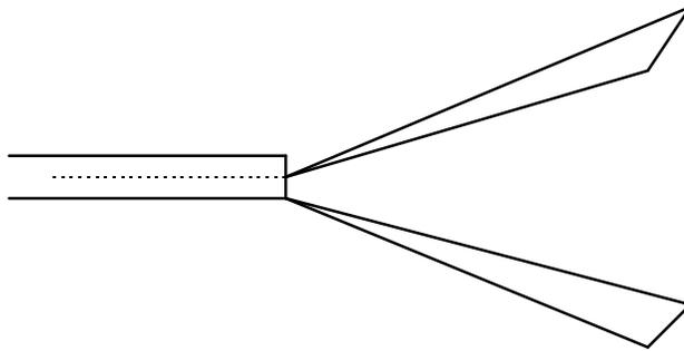
Figure 2.2. A TEM horn fed by a cable.
