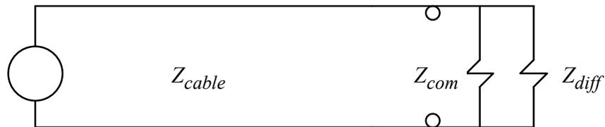
Figure 3.1. Equivalent circuit of the common and differential modes.
