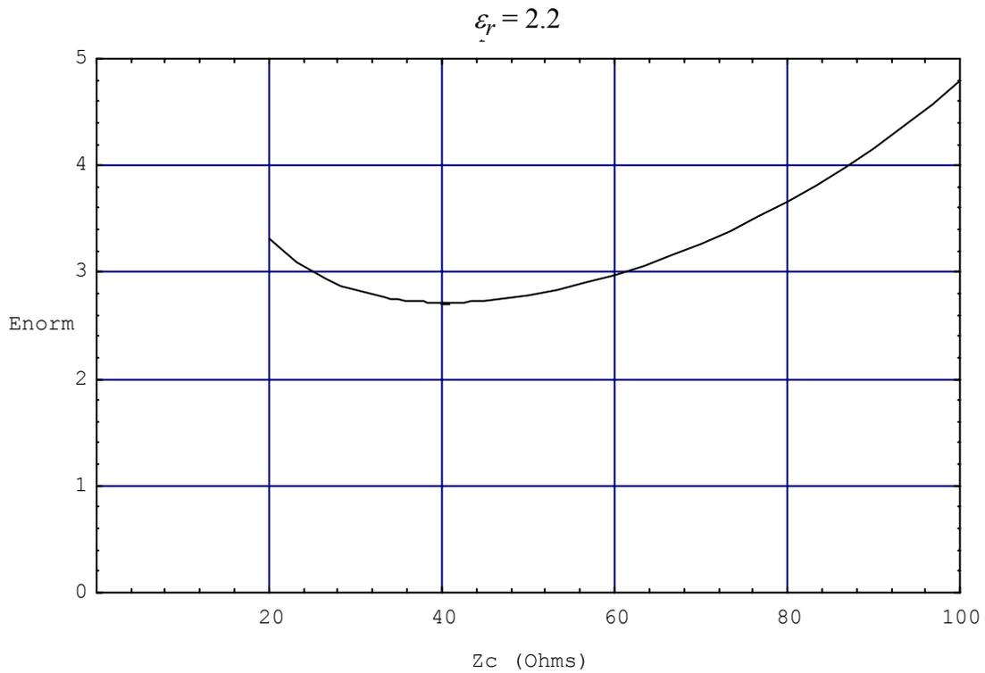
Figure 4.2 Normalized electric field as a function of impedance for  $\epsilon_r = 1$  (top) and for  $\epsilon_r = 2.2$  (bottom). Note the minima near  $Z_C = 40 \Omega$  for  $\epsilon_r = 2.2$  and  $Z_C = 60 \Omega$  for  $\epsilon_r = 1$ .
