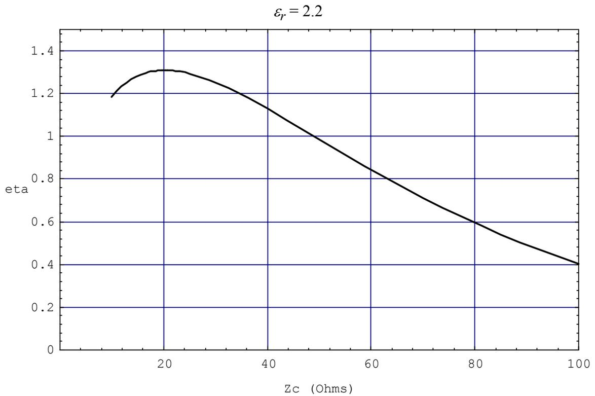
Figure 4.3. Efficiency factor for obtaining high power at low fields  $\epsilon_r = 1$  (top) and for  $\epsilon_r = 2.2$  (bottom). Note the maxima near  $Z_c = 30 \Omega$  for  $\epsilon_r = 1$  and  $Z_c = 20 \Omega$  for  $\epsilon_r = 2.2$ .
