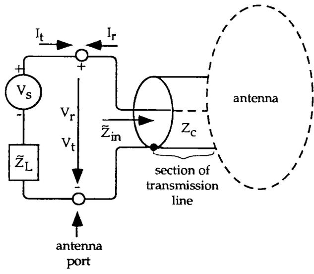
Fig. 1.1. Antenna in Transmission and Reception
