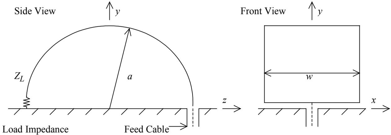
Figure 2.1 Geometry of the BDA.
