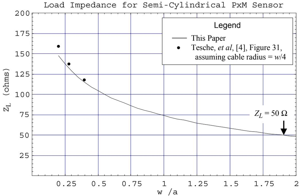
Figure 4.1. Load impedance for a semi-cylindrical P×M sensor as a function of width-to-radius ratio.
