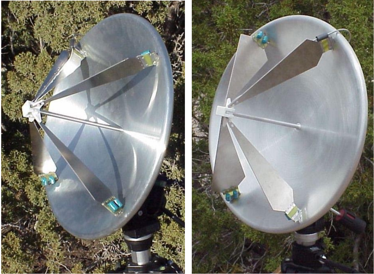
Figure 2.1. IRA-1 with feed arms at \pm 45^\circ (left) and IRA-2 with feed arms at \pm 30^\circ (right).
