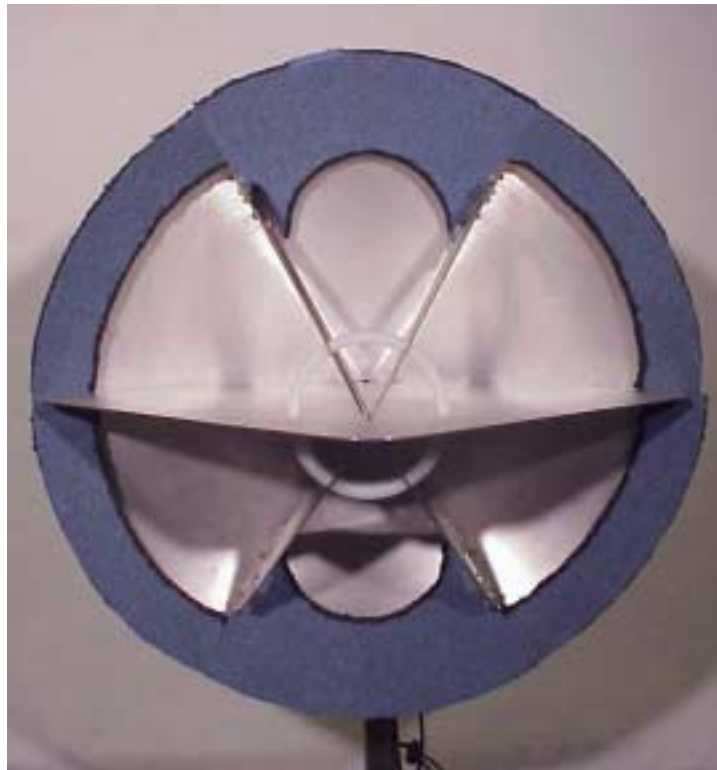
Figure 5.14. IRA-4 with absorber foam around rim.
