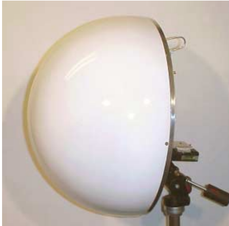
Figure 4.11. IRA-3 with radome manufactured by MRC.
