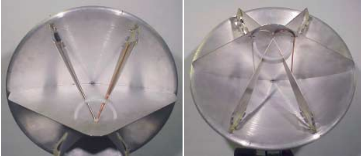
Figure 5.8. IRA-4 with symmetry cables installed.
