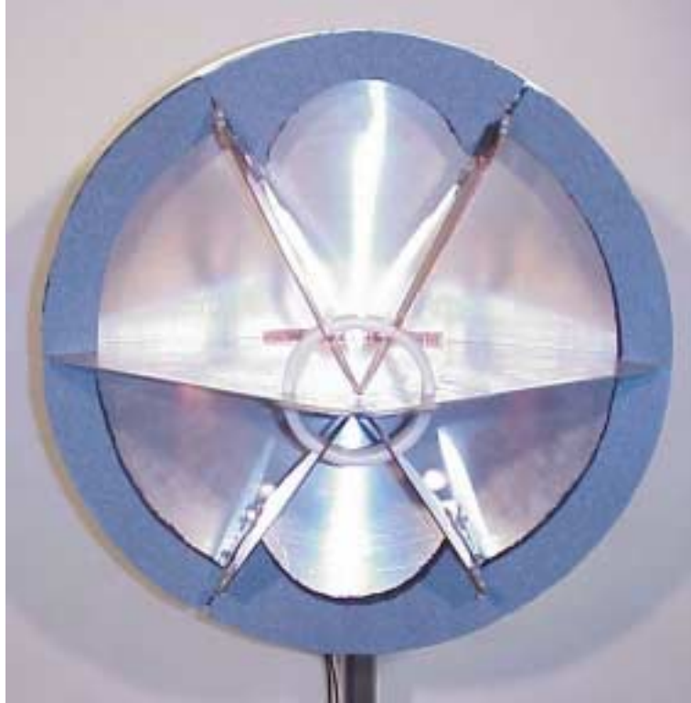
Figure 4.17. IRA-3 with absorber foam.
