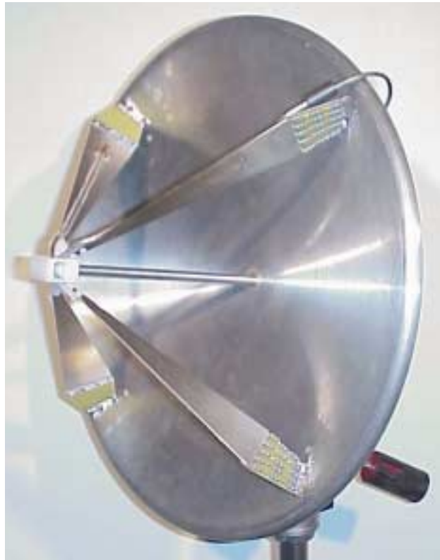
Figure 2.1. IRA-1 (Feed arms at \pm 45^\circ ).
