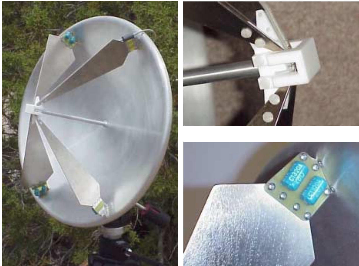
Figure 3.1. IRA-2 (feed arms at \pm 30^\circ ) with feed point and resistor details.
