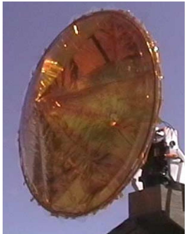
Figure 5.6. Inflated Membrane IRA during RF characterization.
