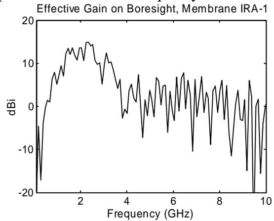
Figure 5.9. Effective Gain of the Membrane IRA.
