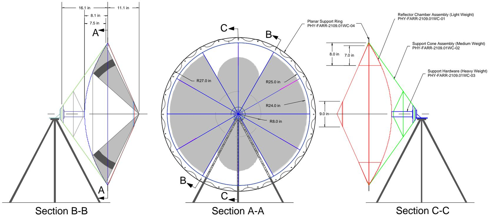
Figure 5.3. Assembly drawing of the Membrane IRA.
