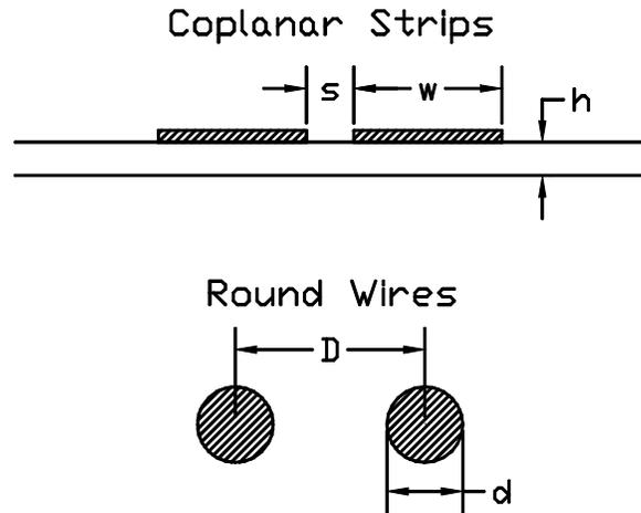
Figure 2.1. Plated twinline (top) and round wires (bottom).
