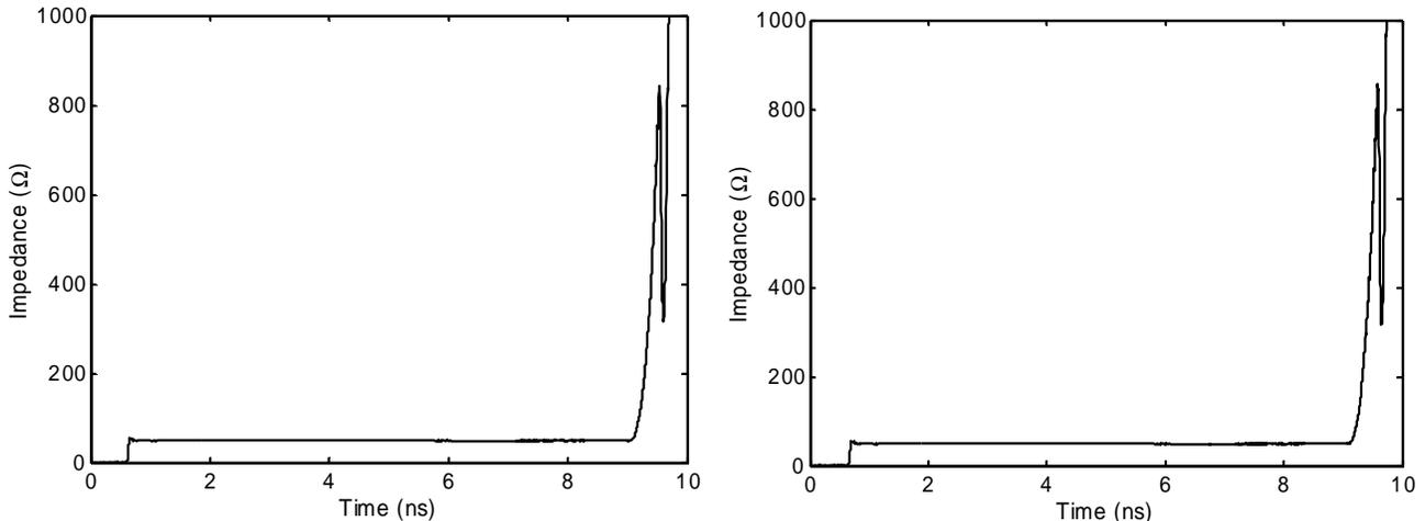
Figure 4.1. Comparison of TDRs with Al on Kapton<sup>®</sup> (left) and 1.6mm (1/16") thick Al Plate (right).
