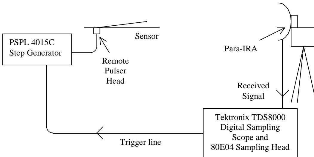
Figure 7.1. Time-domain antenna range measurement system.
