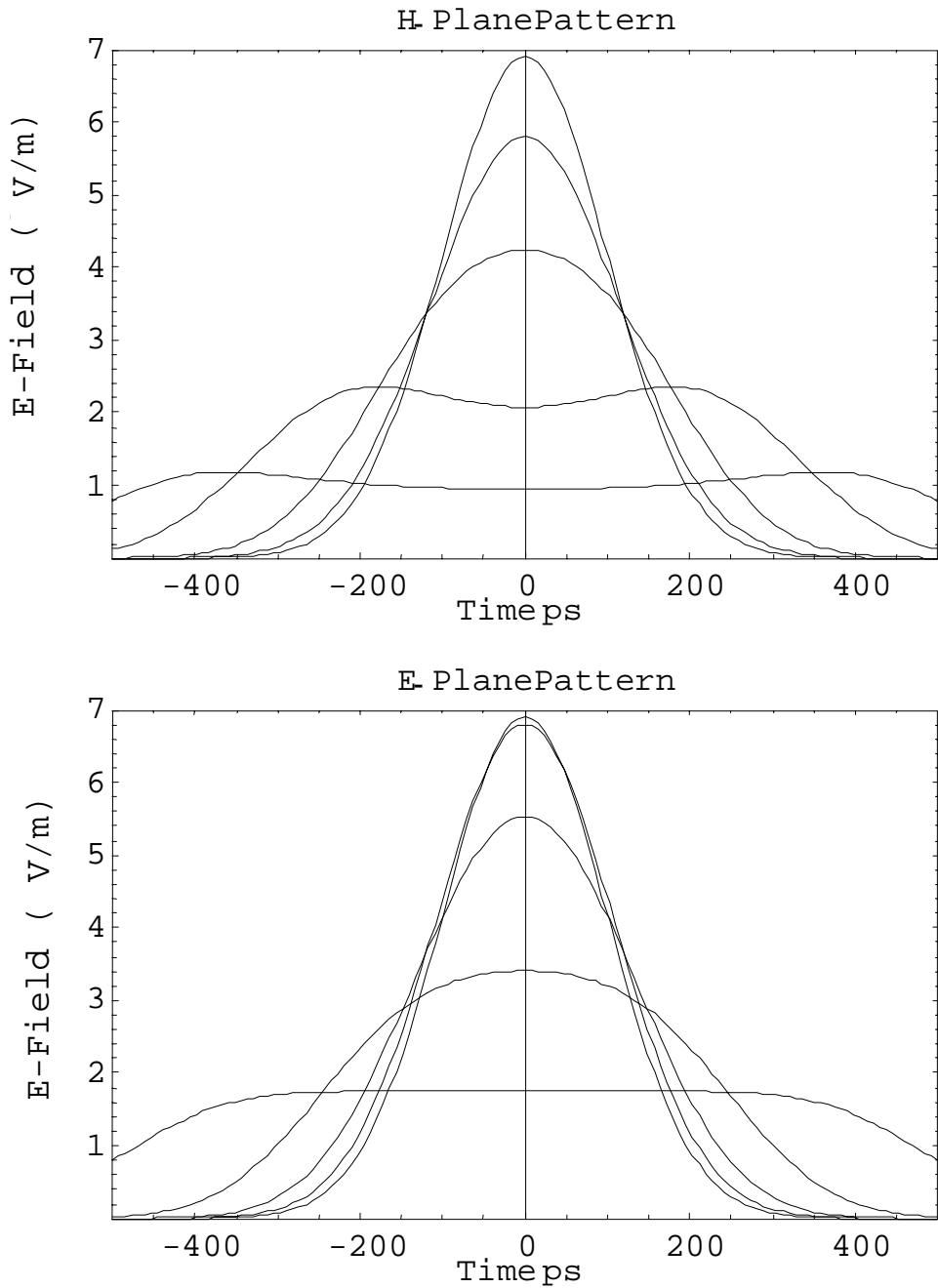
Figure 6.1. Radiated field in the H-Plane (top) and E-Plane (bottom) for the Para-IRA with a 4-foot (1.22 m) diameter, with feed arms at  $\pm 45^\circ$ , observed at a distance of 500 m, driven by a 500 V pulser with risetime of 250 ps.
