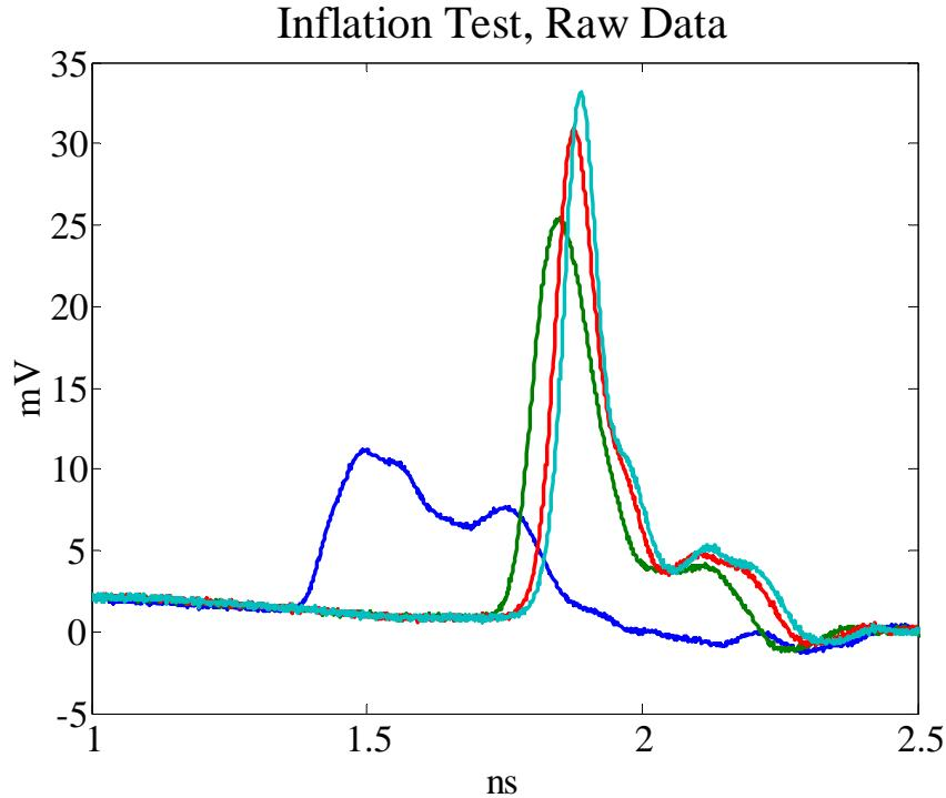
Figure 7.11. Voltage on boresight for inflation test.
