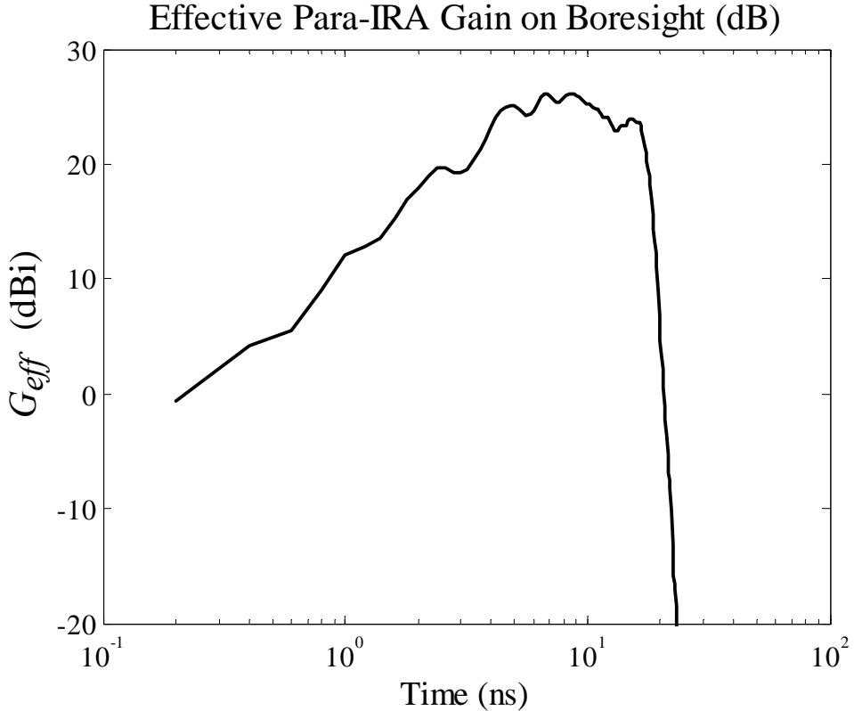
Figure 7.4. Effective Gain of the Para-IRA on Boresight.
