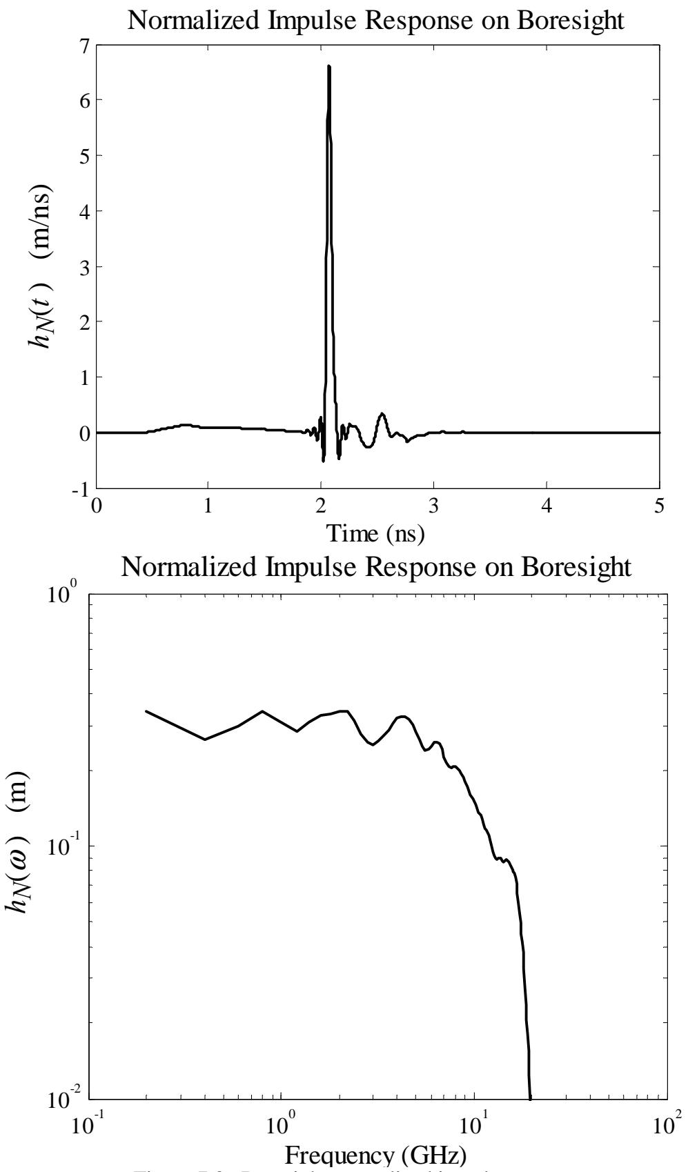
Figure 7.3. Boresight normalized impulse response.
