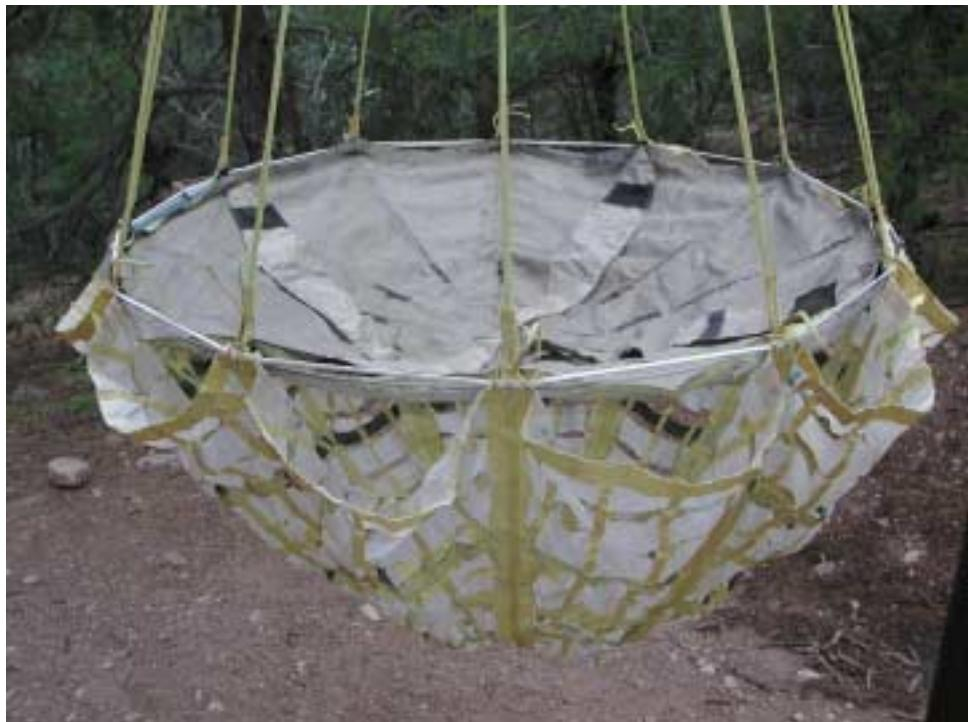
Figure 4.5. Irvin Aerospace's ribbon parachute with mesh CIRA.
