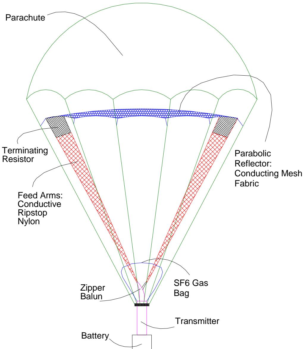
Figure 1.1. Para-IRA with parachute, antenna, balun, SF<sub>6</sub> gas bag, transmitter, and battery.
