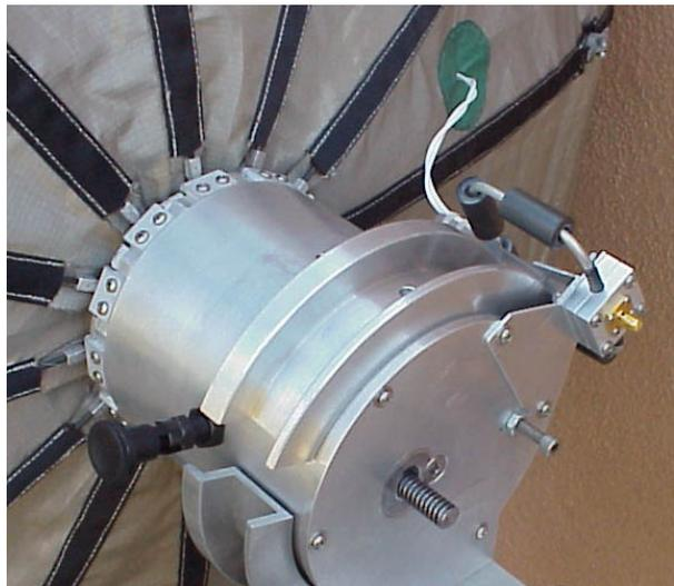
**Figure 2.2 Splitter/Balun (left) and deployment mechanism (right).**
