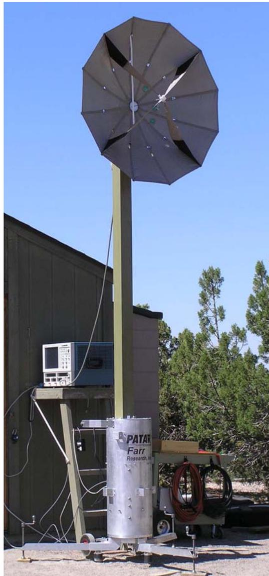
Figure 6.1 RF testing of UCIRA-2 using *PATAR*<sup>TM</sup> system.
